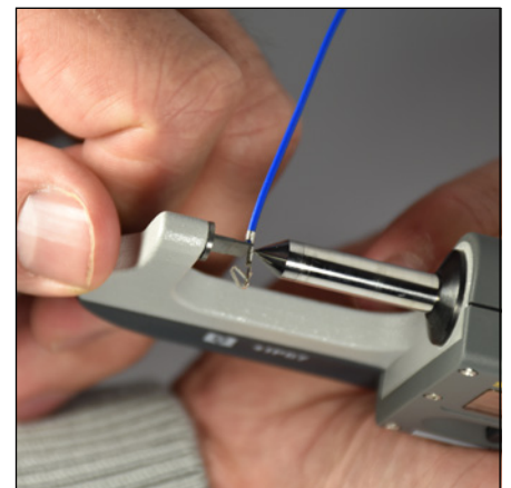
Cable crimping measurement
