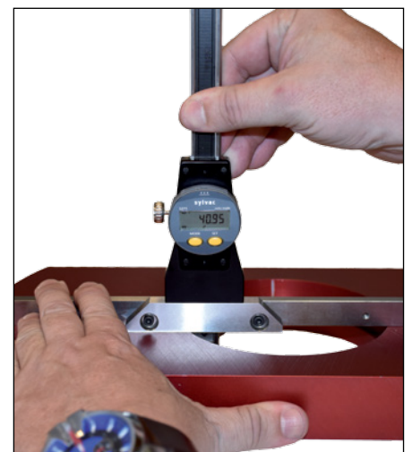
Depth measurement in a drilling with an additional base
