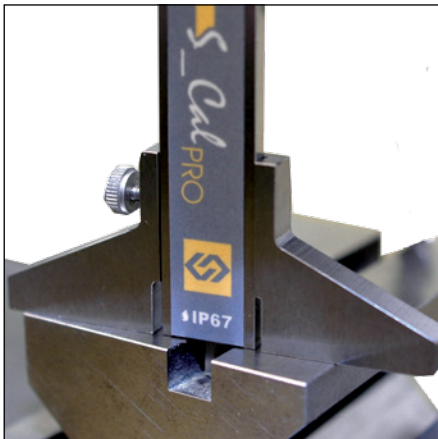
Depth measurement with S_Cal PRO and base 910.2205.
