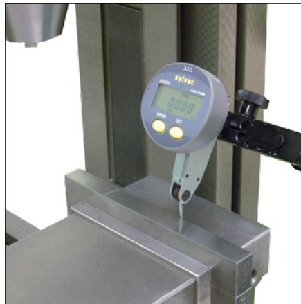
Checking the alignment on milling machine.
